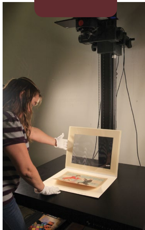
▲ Duplication Services uses this scan stand and camera to digitize items in the Library's collection. Abby Brack Lewis
