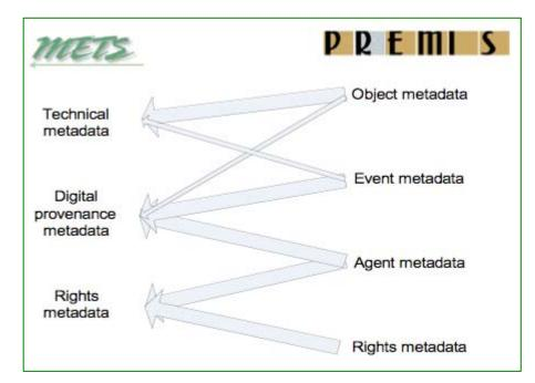
Mapping PREMIS entities to METS metadata sections. Thick arrows show applicable subsection in METS for the named PREMIS entities; the thin arrow shows links from one PREMIS entity to another METS subsection.
